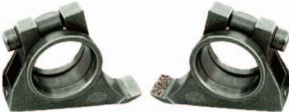
Casted Miehle gripper finger.
