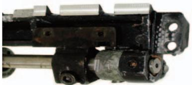
After the aluminum epoxy is dried, the bar is set-up onto a milling machine to machine all pads flat and in line to each other.
