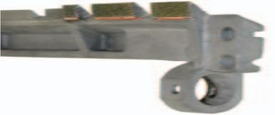
We cut each diamond cover from the copper strip, cutting the sides flush to the diamond coating and leaving about one eighth of inch of copper for the front and back side of pads.
