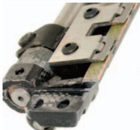
A picture of a Ryobi PFA gripper bar that was reconditioned with a 80/100 grit diamonds. The gripper fingers have the diamond coating bonded on to them and the bar pads have diamond covers glued.
