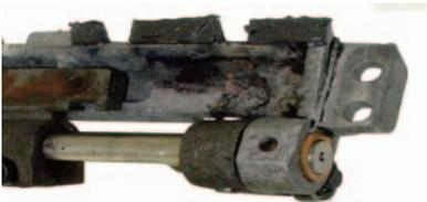
Inspecting each gripping pad surface for low spots, the pads are then cleaned before bonding an aluminum epoxy to build-up the pad surface.
